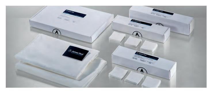
Colour fastness to rubbing is the most basic of colour fastness tests. The dyed sample is rubbed, under controlled conditions, against the white crocking cloth. Subsequently, the degree of colour transfer is evaluated using a Grey Scale for assessing staining.
