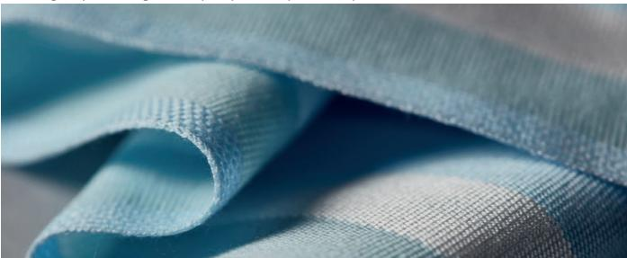
Our internally woven Multifibre LW is approved by a number of UK retailers including Marks & Spencer. It has a similar composition to the Multifibre DW variation but with the acetate strip replaced by the regenerated cellulose strip.
