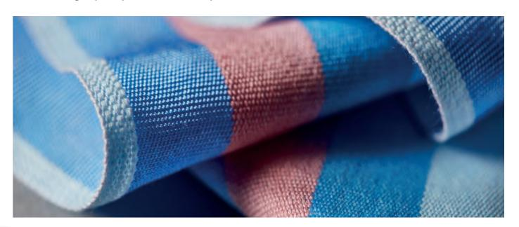
We weave our Multifibre DW internally, carrying out a consistent testing process to ensure you receive a consistently high-quality test fabric. The materials composition is compliant with the requirements specified in ISO 105 F10 and is approved by many leading UK and European specifiers.
