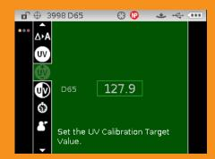
Calibrated UV component – first X-Rite handheld spectrophotometer with adjustable UV component to fully characterize optically brightened
