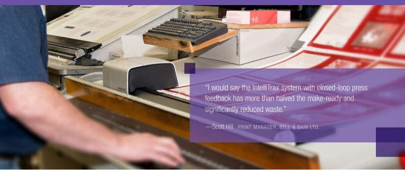
▲ PICTURED: Scan the color bar on a typical press sheet in less than ten seconds.
