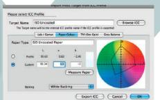
When selecting an ICC profile as the press target you can measure paper color and pressSIGN adjusts the profile. The adjusted profile can be exported for use in proofing etc.
